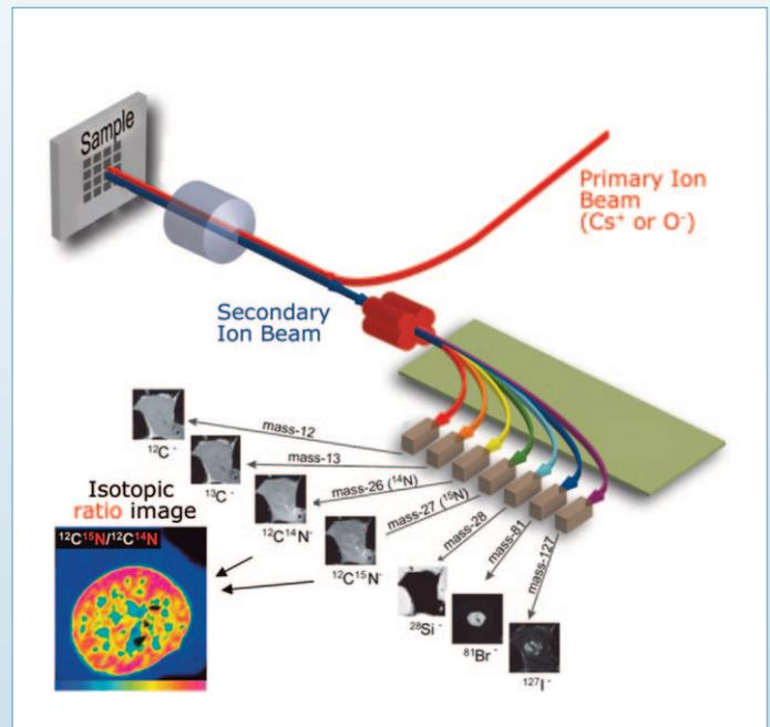
Figure 3: Synoptic of the NanoSIMS 50L secondary ion mass spectrometer.
